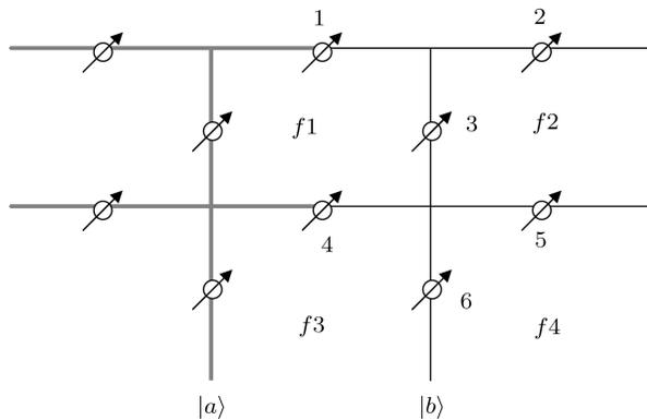
**Fig. 4** The simulation of the CNOT gate. The red part is the control qubit in state  $|a\rangle$  with  $a = 0, 1$ , while the black part is the target qubit in state  $|b\rangle$  with  $b = 0, 1$ .
